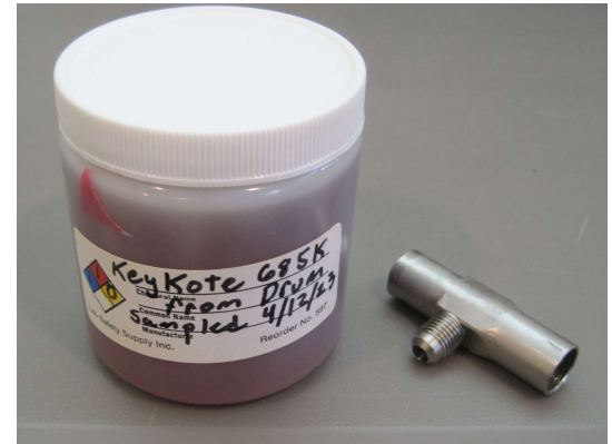
KeyKote 695K oil provided by customer was used to calibrate the UVF-Trilogy for analysis. The oil dissolves instantly in hexane solvent.
