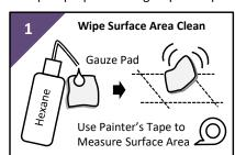
Add hexane to the solvent dispenser squirt bottle. Dampen a gauze pad with solvent and wipe the surface area clean to collect the sample. Surface areas can vary. Testing a small 100x100 mm square surface is typically used. Use a ruler and tape to measure the area to be wiped.
