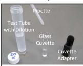
Fill a glass cuvette about half full with the dilution made in Step 3. Pour dilution from test tube into cuvette or use the pipette to transfer dilution into cuvette (less messy). Wipe the outside glass clean using a tissue wipe to remove any liquids or fingerprints. Be careful not to spill cuvette into the cuvette adapter.
