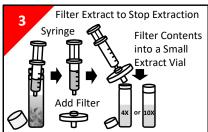
Once the sample has been extracted for 10 minutes, remove the cap, dip a syringe into the vial and suck up the Extract into the syringe. Screw on a filter, push down on the plunger and filter the Extract into a small glass extract vial. Label the vial with "4X" or "10X." Samples extracted for 24 hours will produce higher concentrations and is recommended for coal tar sealcoats
