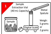
Asphalt samples should be crushed and sieved to 4 mm particle size prior to use following ADEPT (UK) guidelines. Using a glass sample extraction vial, remove the cap and place the vial onto the scale and tare the weight to zero. Scoop out and weigh 5.0 g of sample into the vial. Or use 2.0 g for highly contaminated samples. Be precise (within +/- 0.1 g).
