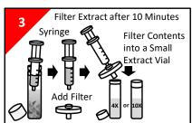
Once the sample has been extracted for 10 minutes, remove the cap, dip a syringe into the vial and suck up the Extract into the syringe. Screw on a filter, push down on the plunger and filter the Extract into a small glass extract vial. Label the vial with "4X" or "10X." Samples extracted for 24 hours will produce higher concentrations and is recommended more for coal tars.
