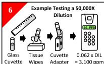
Pour the dilution in Step 5 into a glass cuvette, place into the analyzer and press the READ button. Multiply the reading by the dilution factor to report the final concentration.
