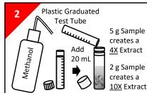
Add methanol to the solvent dispenser bottle. Squirt 10 mL of methanol into a plastic graduated test tube. Pour contents into the sample extraction vial. Add another 10 mL to vial for a total of 20 mL of solvent. Keep track of the dilution created in the extract (4X or 10X). Tighten cap and shake vial periodically for 10 minutes, no more than 20 minutes.
