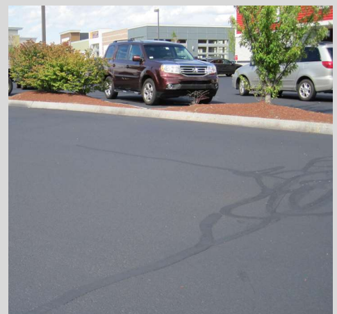
Avoid collecting samples where cars are parked or where crack fillers have been used previously. Drippings from motor oil or wear from tires may contain hydrocarbons which will interfere with the sealcoat test results.
