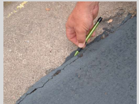
The interface where the sealcoat meets concrete or the edges of a parking lot is a good location to find and collect samples.
