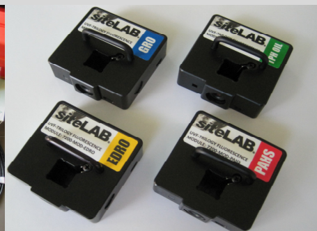
Fluorescence UV Modules are fitted with LEDs and optical filters sensitive and selective to different types of hydrocarbons
