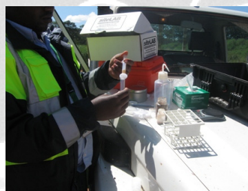
Soils are field screened for Total Petroleum Hydrocarbons (TPH).
