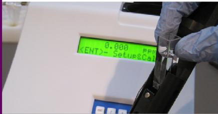
Metal samples are extracted in solvent and measured on the analyzer. The concentration of oil is displayed in ppm units. Test results can be converted to mg/m<sup>2</sup> if the surface area is known, which is often required for certain applications.
